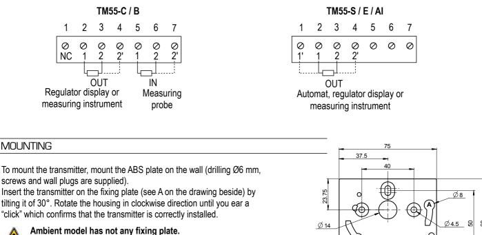
4 fixing holes are inside the back housing. Use them to install the transmitter on the required location. The contact model is fixed with 2 mounting brackets supplied with the transmitter.
