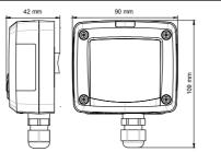
Contact type and model with terminal block
