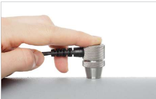
Wall thickness gauge NT in use
