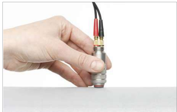
Wall thickness gauge HT in use
